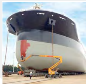
Painting & Blasting system • Painting hull ship • Abrasive steel blasting inside tanker
